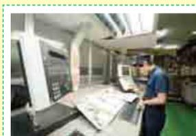
5 Small stains and dirt are detected using a high performance camera. A visual check is also conducted. An operator checks the color tone and dirt by looking at the colored proof, and modifies and adjusts the color.
