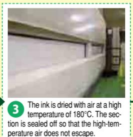
3 The ink is dried with air at a high temperature of 180°C. The section is sealed off so that the high-temperature air does not escape.
