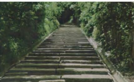
The stairs of Kensoji Temple in Azabujuban before restoration. These stairs were built by the Nabeshima clan during the Edo period. The depths of each step is one step and a half with only a small difference in level so as to minimize tilting of the large palanquin carrying the lord.
