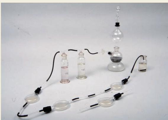
Kitasato’s invention: Anaerobic bacteria culturing equipment (model)*
