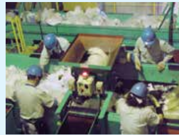
Tearing garbage bags and removing unrecyclable objects
