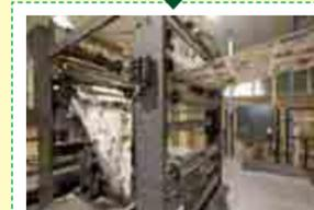
6 Folding Process and Cut-out It is just like a giant weaving machine! Paper is simultaneously drawn into the machine and folded.
