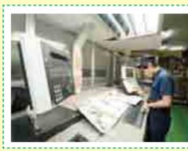
5 Small stains and dirt are detected using a high performance camera. A visual check is also conducted. An operator checks the color tone and dirt by looking at the colored proof, and modifies and adjusts the color.
