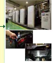
Magenta (M) and Yellow (Y) are applied in turn to the print. Simultaneous printing of the front and reverse sides is performed
